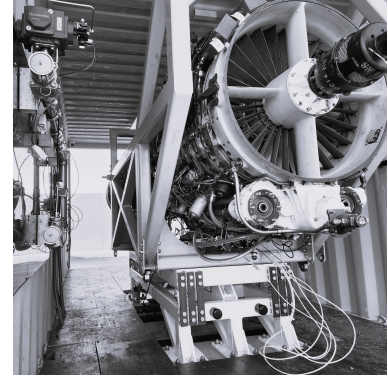
Figure 6: SES’ engine test cell with engine installed.
