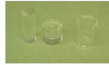
Sapphire mortar and pestle for ultra clean U-Pb work
