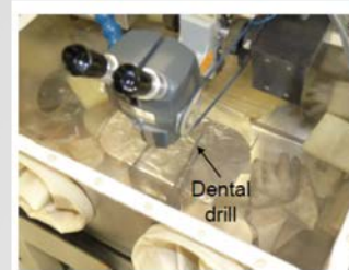
Extract sample (using dental drill)
