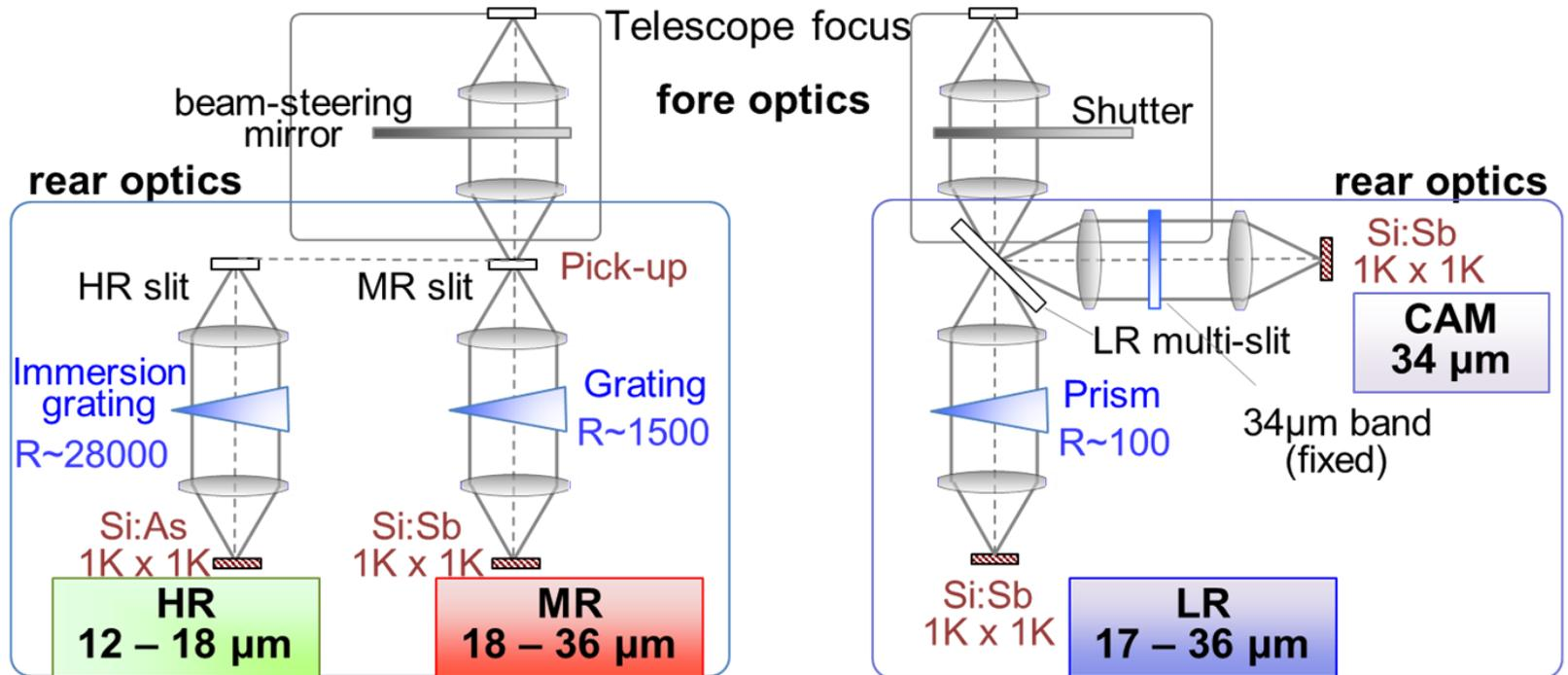
**SMI / LR-CAM:** Multi-slit prism + Si:Sb w/ 10'x12' slit viewer
